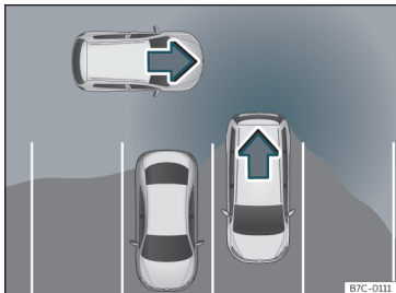
Fig. 224 Diagram of the parking assistant: detected area around the vehicle that is driving off.
