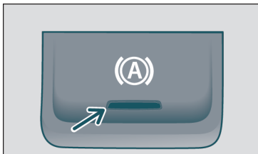
Fig. 201 In the lower part of the centre console: Auto Hold function button.
