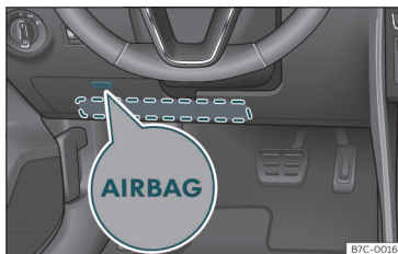
Fig. 24 On the driver side: location of airbag for knees.
