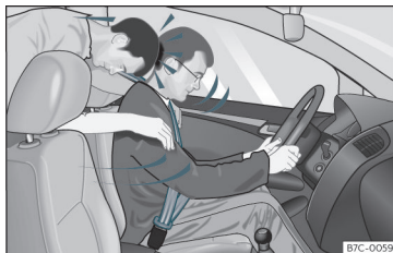
Fig. 78 The unbelted passenger in the rear seat is thrown forward violently, hitting the driver who is wearing a seat belt.
