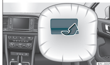
Fig. 21 Front passenger airbag located in dash panel.
