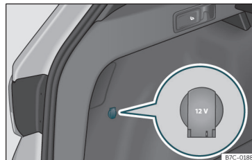
Fig. 134 Detailed view of the side trim in the boot: 12-volt power socket.
