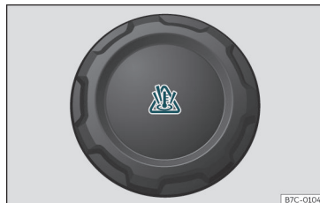
Fig. 51 Engine compartment: coolant expansion tank cap.
