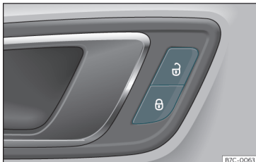
Fig. 2 Driver door: central locking switch.
