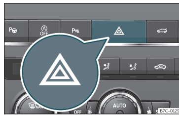
Fig. 39 Dashboard: switch for hazard warning lights.
