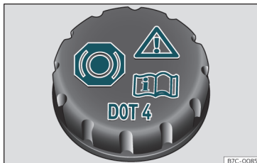
Fig. 52 Engine compartment: brake fluid reservoir cap.
