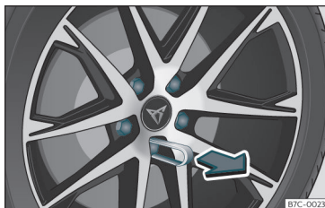
Fig. 59 Wheel: wheel bolts with caps.
