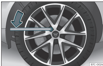
Fig. 61 Wheel: loosen the wheel bolts.
