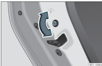
Fig. 113 Childproof lock on the left hand side door.
