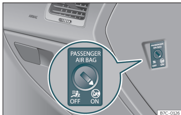
Fig. 22 Front passenger front airbag switch.
