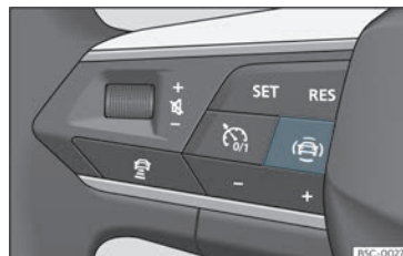
Fig. 62 Left side of the multifunction steering wheel: button for assistant systems (depending on versions).
