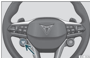
Fig. 144 Multifunction steering wheel*: button to change the driving profile.
