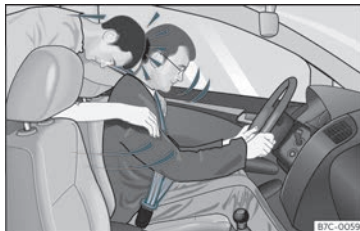
Fig. 8 The unbelted passenger in the rear seat is thrown forward violently, hitting the driver who is wearing a seat belt.
