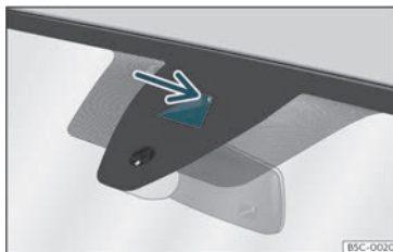
Fig. 147 On the windscreen: field of vision of the Lane Assist system.
