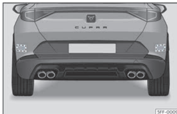
Fig. 148 Rear view of the vehicle: radar sensor zones.
