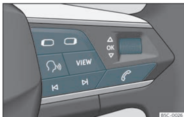
Fig. 60 Right side of the multifunction steering wheel: buttons for using the instrument cluster's menus and information displays (depending on versions).
