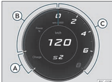
Fig. 57 Digital instrument panel: Powermeter (Cupra view)
