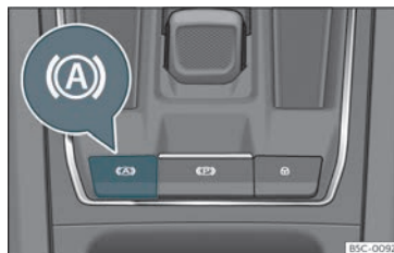
Fig. 173 In the lower part of the centre console: Auto Hold function button.
