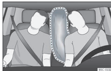
Fig. 20 Fully inflated central airbag (deployment zone).
