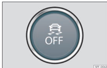
Fig. 174 In the lower part of the centre console: button to switch the ESC off/on
