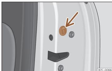
Fig. 85 Locking the door manually.
