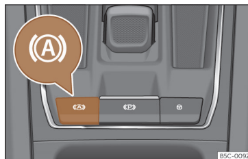
Fig. 190 In the lower part of the centre console: Auto Hold function button.
