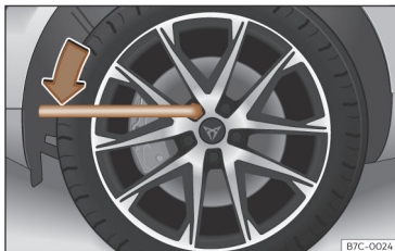
Fig. 42 Wheel change: loosen the wheel nuts.
