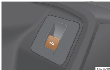
Fig. 89 On the driver's door: button to open and close the rear lid.
