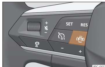
Fig. 67 Left side of the multifunction steering wheel: button for driver assistance systems (depending on versions).
