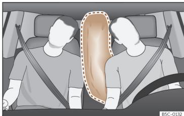
Fig. 24 Fully inflated central airbag (deployment zone).
