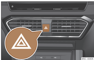
Fig. 98 Dash panel: hazard warning lights switch
