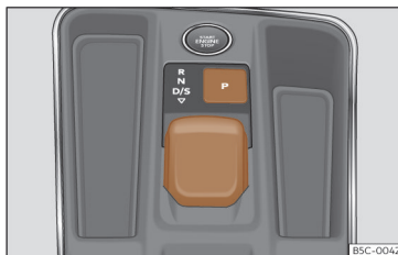
Fig. 159 In the centre console: selector lever.
