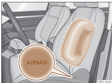
Fig. 25 Side airbag in driver's seat.
