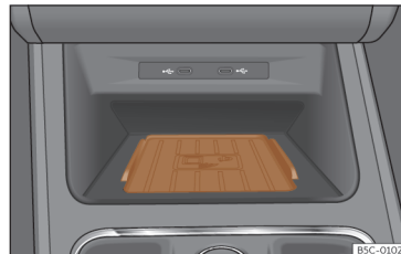
Fig. 153 In the centre console: pad for the mobile phone connection.
