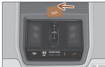
Fig. 36 On the roof console: voice service controls
