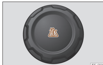
Fig. 226 Engine compartment: coolant expansion tank cap.
