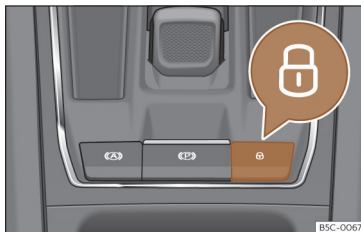
Fig. 81 In the centre console: central locking switch
