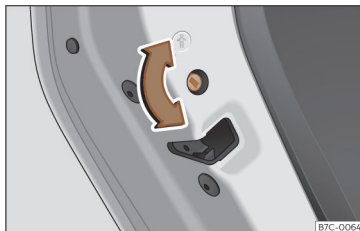
Fig. 86 Childproof lock on the left hand side door.
